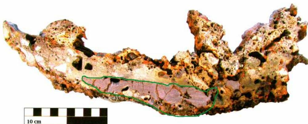
*Fig. 7: Section through the mass of slag, where the matte can be seen at its bottom (outlined in green). The upper part of the slag is characterized by being very porous with inclusions of charcoal, and pieces of quartz, which is also typical of the prehistoric slag cakes.*
