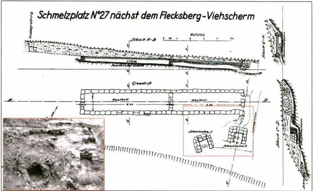
Fig. 1: Plan and photo of smelting site "27", Mitterberg, Mühlbach am Hochkönig, Austria. A: Roasting Beds. B: Furnaces.
