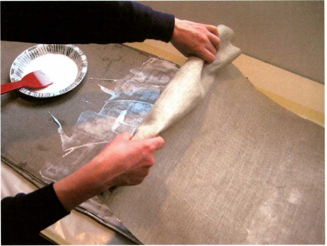
Fig. 3: Laminating layers of fabric together.
