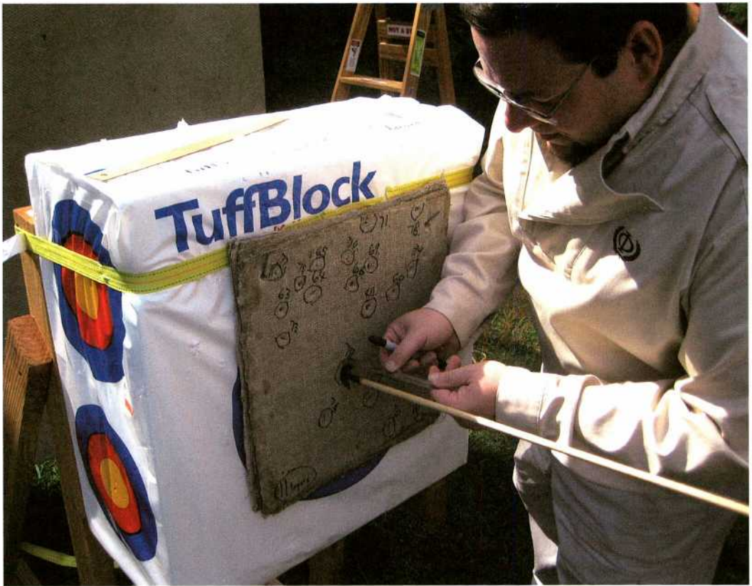
Fig. 5: Measuring penetration of arrow into test patch.
