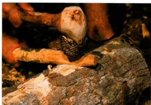
Fig. 4: Fabrication of a pointed stick: rough-hew.
